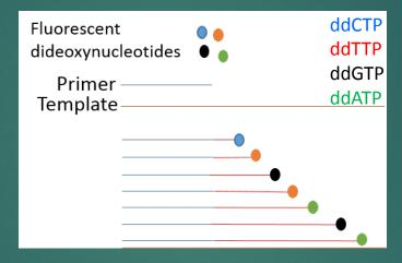
3. Products are separated by size; fluorescent tags detected by laser. Chromatogram output analyzed by software.
